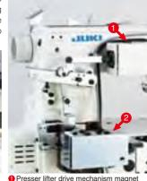
2 Thread trimmer drive mechanism magnet
