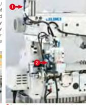
Presser lifter drive mechanism air cylinder 2 Thread trimmer drive mechanism air cylinder
