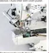
Electromagnetic needle thread / looper thread trimming device
