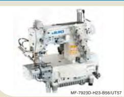
This model is best suited to hemming processes for sleeves and the bottoms of T-shirts, Polo shirts, etc. It comes with a left hand fabric trimmer for trimming fabric in parallel, at all times, to the seam with consistency. The upper knife stroke can be adjusted with ease.
