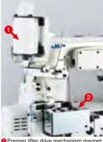
Presser lifter drive mechanism magne 2 Thread trimmer drive mechanism magnet
